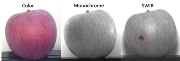
**Figure 5 — When fruit is bruised, the cell walls break down and the area develops a higher moisture content. Water absorbs many bands of light in the SWIR range. This absorption allows SWIR imaging to see bruises that aren't detectable by visible camera technologies.**
