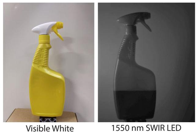
**Figure 6 — A 1550 nm SWIR light can enable a SWIR camera to see through a plastic container and show the fluid level.**
