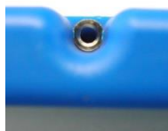
Figure 3. Correctly installed insert
