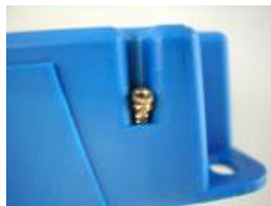
Figure 1. Insert at bottom of slot ready to be pushed in
