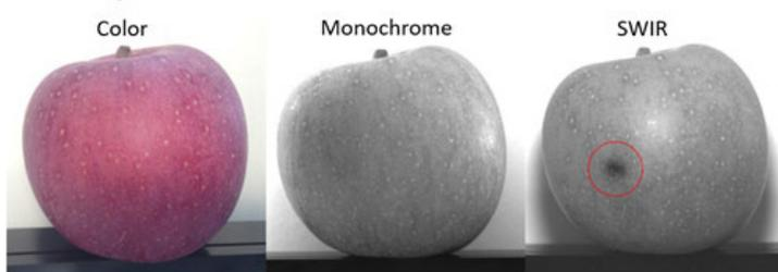
**Figure 5 - When fruit is bruised, the cell walls break down and the area develops a higher moisture content. Water absorbs many bands of light in the SWIR range. This absorption allows SWIR imaging to see bruises that aren't detectable by visible camera technologies.**
