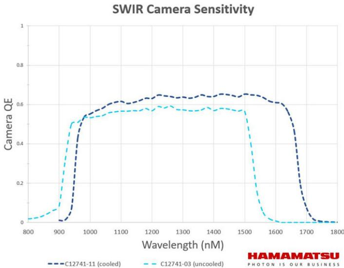
Figure 2 - Typical InGaAs SWIR Camera Performance
