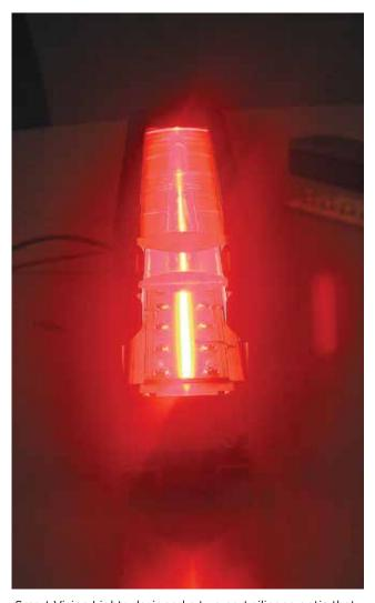
Smart Vision Lights designed a two part silicone optic that can also accommodate a wire polarizer in its new LHP, ultra high-power line light. The light generates 5 million lux, and only silicone optics could withstand that heat without significant degradation over time.
