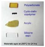
Typical organic materials used for optical systems in lamps and luminaires, and silicone resin aged at 200oC for 24 hours
