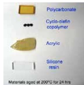
Typical organic materials used for optical systems in lamps and luminaires, and silicone resin aged at 200°C for 24 hours
