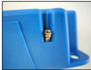
Fig 1. Insert at bottom of slot ready to be pushed in
