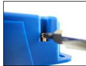
Fig 2. Pushing insert into Housing
