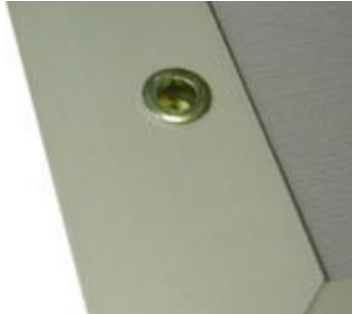
Threaded inserts in aluminum frame
